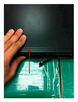
Put the HDD tray back in the case and insert it completely.
